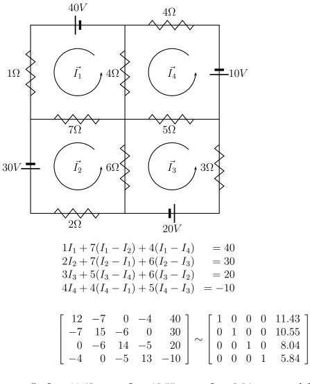
So  $I_1 = 11.43$  amps,  $I_2 = 10.55$  amps,  $I_3 = 8.04$  amps, and  $I_4 = 5.84$  amps.
